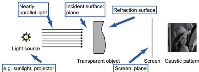
Fig. 2. An illustration of the proposed display system.
