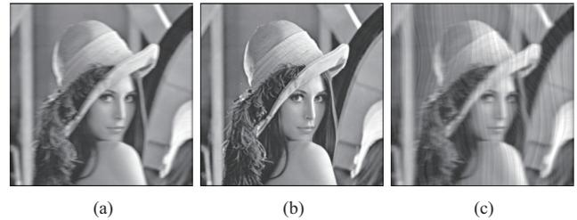
Fig. 15. Simulated caustics taking into account bumps in the refractive surface. The radius of the end mill was 0.5mm in each case. The pitch of the milling path was set to: (a) 0.02mm, (b) 0.005mm, and (c) 0.02mm. In (c), deviations in the paths in the  $z$  direction are taken into account and are modeled using white noise.
