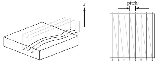
Fig. 13. Left: an illustration of the milling path. Right: a top view. Paths shown in black color are for milling the surface and those shown in gray color are “subsidiary” paths, each of which is used to position the end mill to the next section without touching the surface (the end mill goes up, then moves to the next starting position straightly and horizontally, and then goes down).
