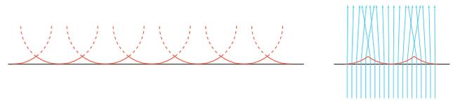
Fig. 14. Left: an exaggerated illustration of a cross-section through the refractive surface (black line) and the fabricated surface (red line) due to the finite radius of the end mill (the materials milled out by the end mill are shown as dashed red lines). Right: an exaggerated illustration of the light refraction with respect to the fabricated surface.
