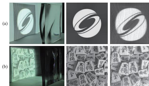
Fig. 11. From left to right: photographs of the fabricated objects and their caustics, the simulated caustic patterns, and the caustic patterns of the fabricated objects.
