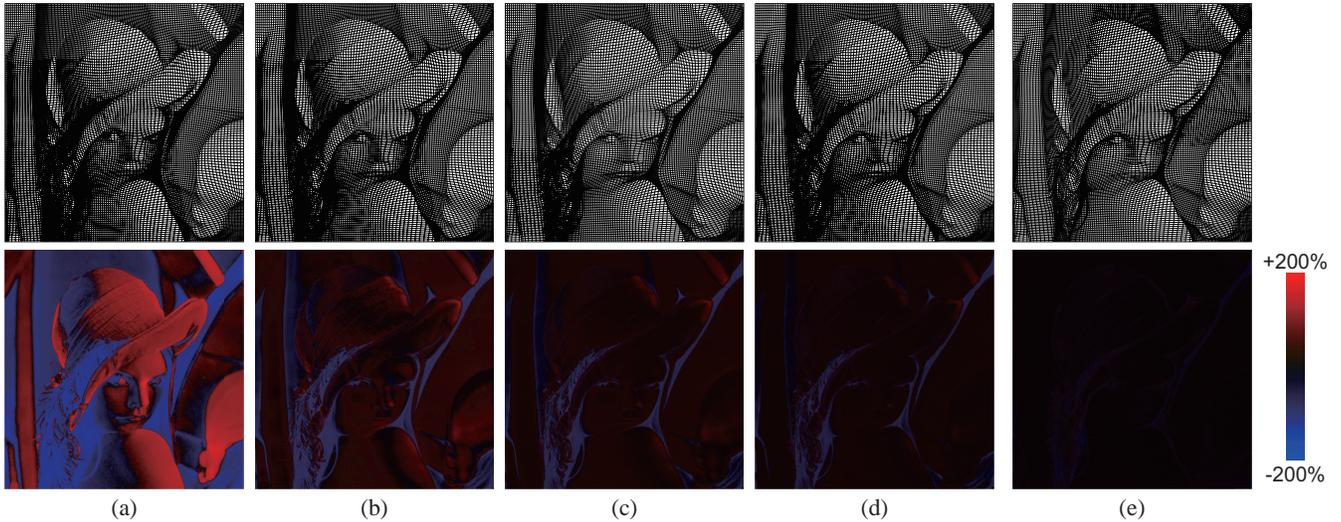
Fig. 6. Computation of the relationship. (a) to (e): Results after 1, 3, 5, 7 and 25 steps, respectively. The top row shows the isoparametric lines for displaying the parameterization (please enlarge the figure to see the details). The bottom row shows the difference  $D$  (red and blue portions indicate positive and negative regions, and the difference is normalized such that the average intensity of the desired caustics corresponds to 100%).
