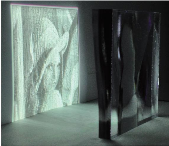
Fig. 1. The fabricated object (right) and its caustics (left) on the screen. Please see Figure 7 for the shape of the refractive surface of the object.
