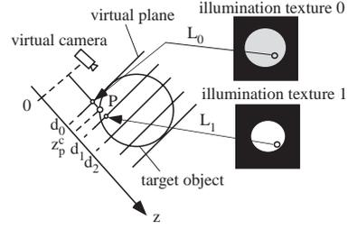
Figure 5: Rendering caustics using illumination textures.
