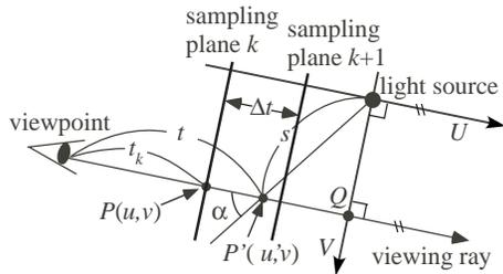
**Figure 2:** Creating the textures for light beams.
