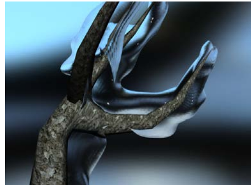
Fig. 8: Simulation result of glazed frost adhering on the windward side by the wind from right to left.
