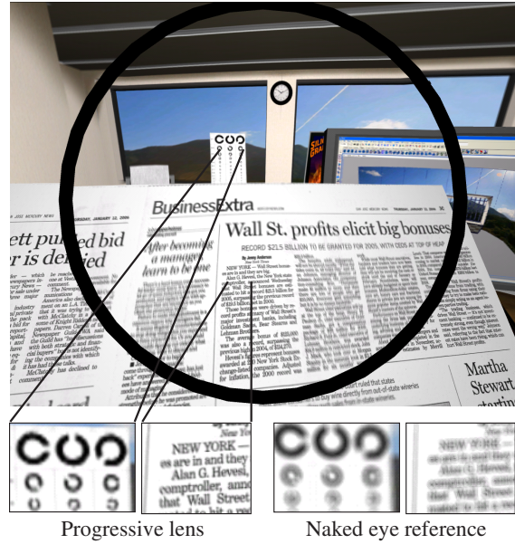
Figure 11: Correction by a prototype progressive lens.
