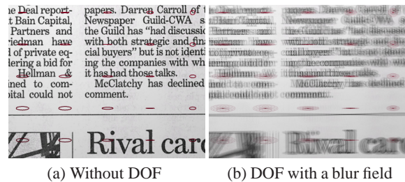
Figure 12: An astigmatic naked eye simulation result. The newspaper object is placed so close (6.1cm at the lower-left corners and 10.7cm at the upper-right) that the eye is unable to accommodate. A partial blur field (voxels of almost the same depth as the newspaper) is visualized as an ellipsoid for each voxel. Note that every blur field ellipsoid is also blurred exactly by its own spread range. Also note that the ellipse shapes differ by their distances from the viewpoint, exhibiting the sections of the Sturm's conoid.
