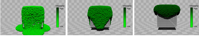
Figure 4: Motion comparison of fluids with different extension coefficients. \beta = 1.005, 1.003, and 1.001 from left to right. Particles are colored according to their viscosity values (low viscosity: light green, and high viscosity: dark green).
