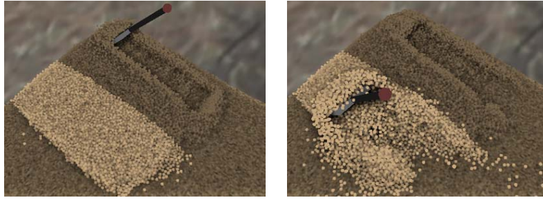
Figure 8: Interaction between granular particles with a rigid shovel.
