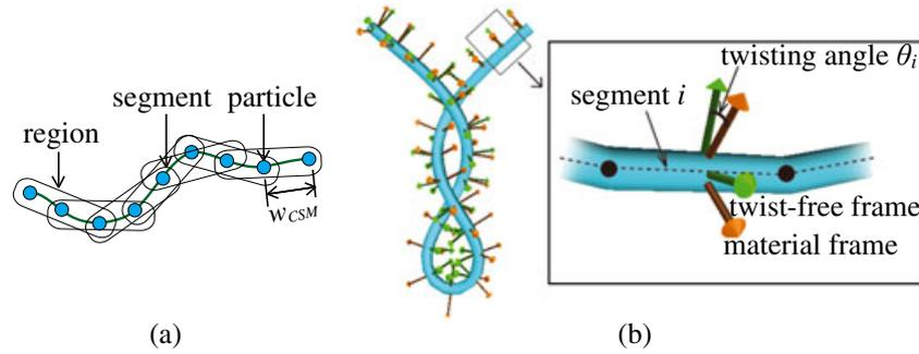
**Figure 1.** Our string model: (a) multiple overlapping chain regions in the chain shape matching; (b) the twisting angle of a segment of an elastic string is an angle between a twist-free frame and a material frame.
