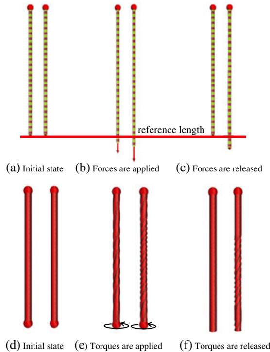
**Figure 8.** Plasticity of the material under tensile and torsional stresses. (a) and (d) are the states before forces and torques are applied in (b) and (d), respectively. In (b) and (d), the strings on the left do not pass the yield points, whereas the strings on the right do. (c) and (e) are the states after the forces and torques are released.
