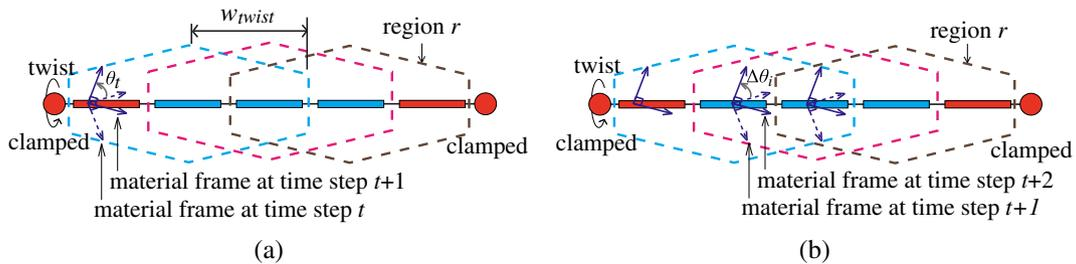
**Figure 2.** (a) An elastic string clamped at both ends is twisted at one end with a twisting angle  $\theta_t$ . (b) The increment of the twisting angle is propagated to the next segments.
