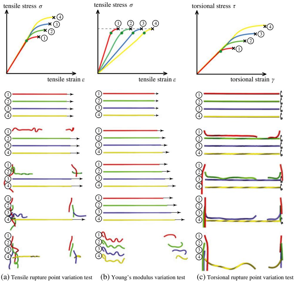
**Figure 7.** Experiments of various stress–strain curves and results of curves. A variety of stress–strain curves are shown at the top row, and their results are shown as animation sequences from top to bottom. (a) Tensile rupture point variation test; (b) Young's modulus variation test; and (c) torsional rupture point variation test.
