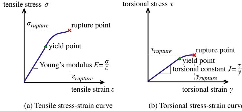
**Figure 3.** Typical tensile and torsional stress–strain curves of a material: (a) tensile stress–strain curve; (b) torsional stress–strain curve.
