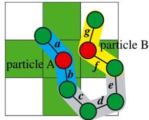
**Figure 5.** A two-dimensional illustration of our optimized searching scheme. When performing a collision detection between Particles A and B, segment collision tests between  $\{a, g\}$ ,  $\{b, f\}$ ,  $\{b, g\}$ , and  $\{b, f\}$  capsules are tested.
