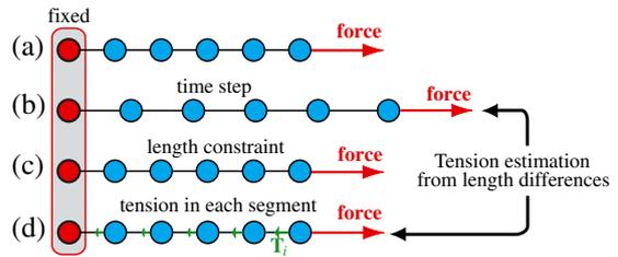
**Figure 4.** A simple example of the tension computation. From (a) to (c), an ordinary length-constrained string simulation is performed. In (d), tensions are estimated by calculating forces that make the particles move from their unconstrained positions to the constrained positions, yielding a result equivalent to (c).
