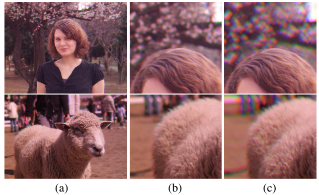
Figure 16: More color misalignment cancellation results. (a) Restored images. (b) Closeups of (a). (c) Closeups of the original.
