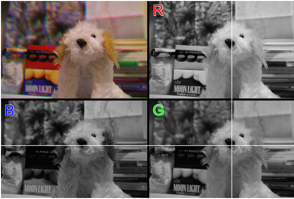
Figure 4: Example photograph taken with our lens, and its separated RGB planes. The white lines are superimposed to highlight the background color shifts. See Fig. 15(a) for a closeup view.
